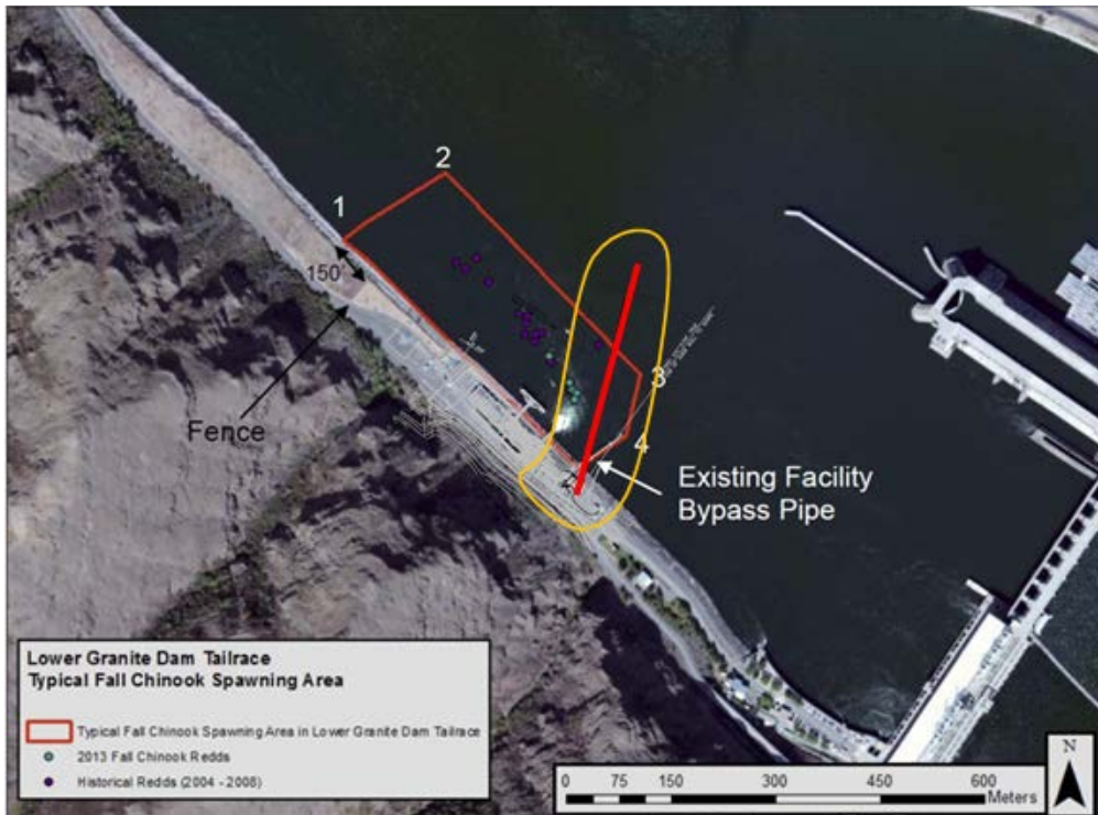
Figure 4. Typical fall Chinook spawning area in the Lower Granite Dam tailrace (area circled in dark red) and new primary bypass outfall construction area (area circled in yellow). The emergency bypass outfall will be constructed upstream of the existing facility bypass pipe where there has been no record of chinook spawning efforts.
